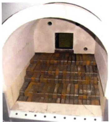
Moveable grate system to burn special fuels (agri waste, contaminated fuel and high ash content)
