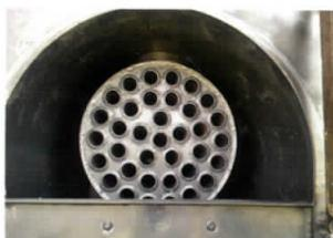
Cylindrical heat exchanger with fire-tubes
